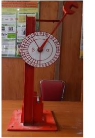
**Figure 4.** Impact testing: Charpy impact test equipment and the specimen
